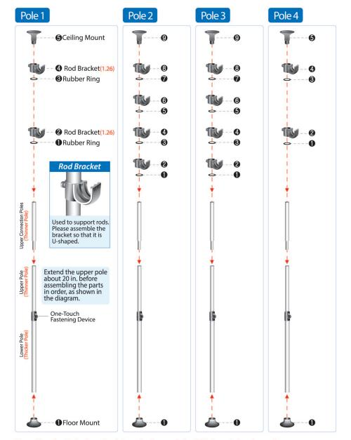
The rubber ring helps keep the fixtures in place and should be inserted underneath each rod bracket. (The rubber rings inserted underneath the rod brackets are not visible after installation.)
