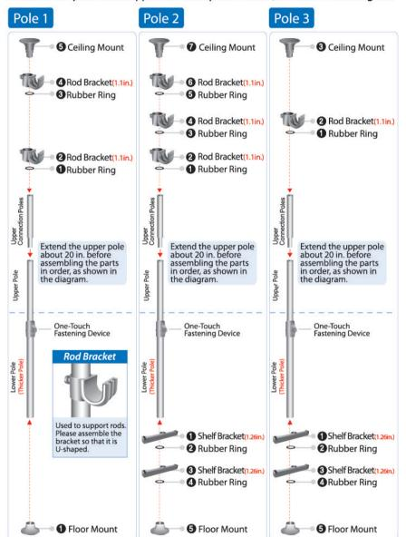
The rubber ring helps keep the fixtures in place and should be inserted underneath each fixture.
