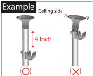
Assemble the fixtures (shelf brackets, rod brackets, etc.) at least 4 in. away from the ceiling mount for firm support.
