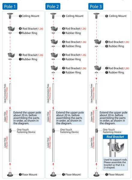
The rubber ring helps keep the fixtures in place and should be inserted underneath each rod bracket.
