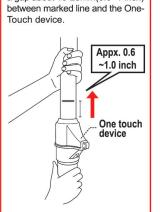
•If the marked line is too low or is not visible, pull the upper pole against the ceiling firmly to check if it is assembled properly.
