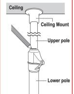
[Figure 2] Push the upper pole to the ceiling as hard as you can. Make sure to have a gap about 15-25mm(0.6~1 inch)
