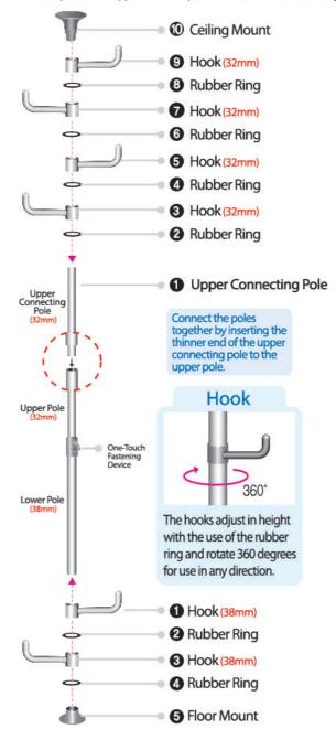
The rubber ring helps keep the fixtures in place and should be inserted underneath each rod bracket. (The rubber rings inserted underneath the rod brackets are not visible after installation.)
